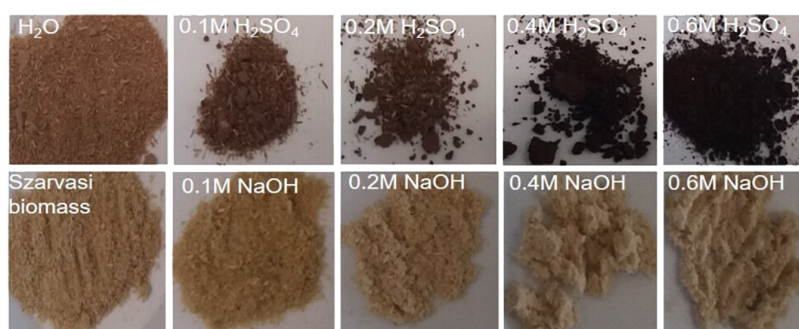
FIGURE 1 | Szarvasi biomass and pulps after various microwave pretreatments including alkaline (NaOH), near neutral (H 2 O), or acidic pretreatments (H 2 SO 4 ).
